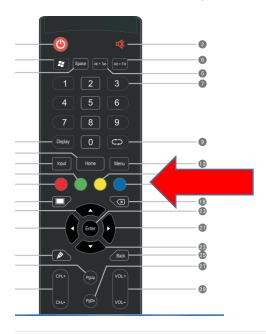
**(**): Press this button to enter standby when power is on; Click this button to switch on in standby condition
